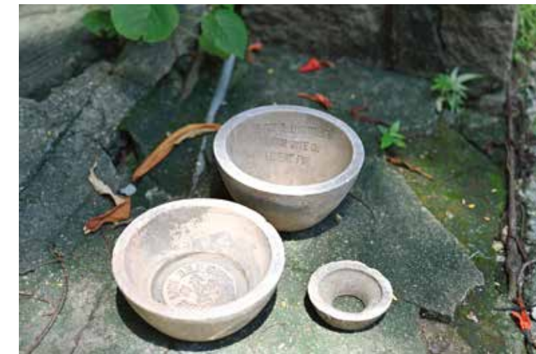
五加皮酒樽模具分為三個部分。 The ng ka py bottle was made from a 3-part mould.
