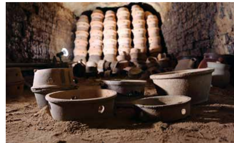
匣鉢疊至窯腔頂部。 Saggars stacked to the kiln ceiling.
