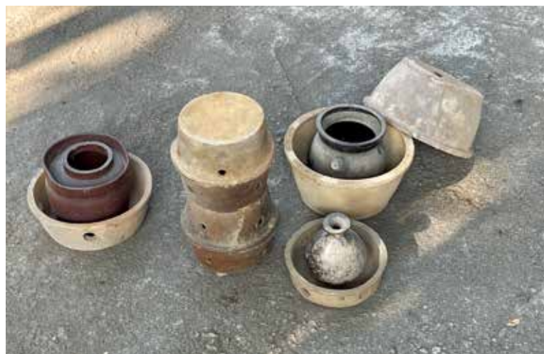
右 工合陶窯備有大小不同的匣鉢。 L Saggars protected the products during firing, and could be stacked to make maximum use of kiln space. R Kung Hop's saggars came in several sizes.
